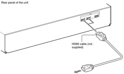
To the HDMI OUT jack of the set-top box/ digital satellite receiver or PLAYSTATION<sup>®</sup>3, etc.
